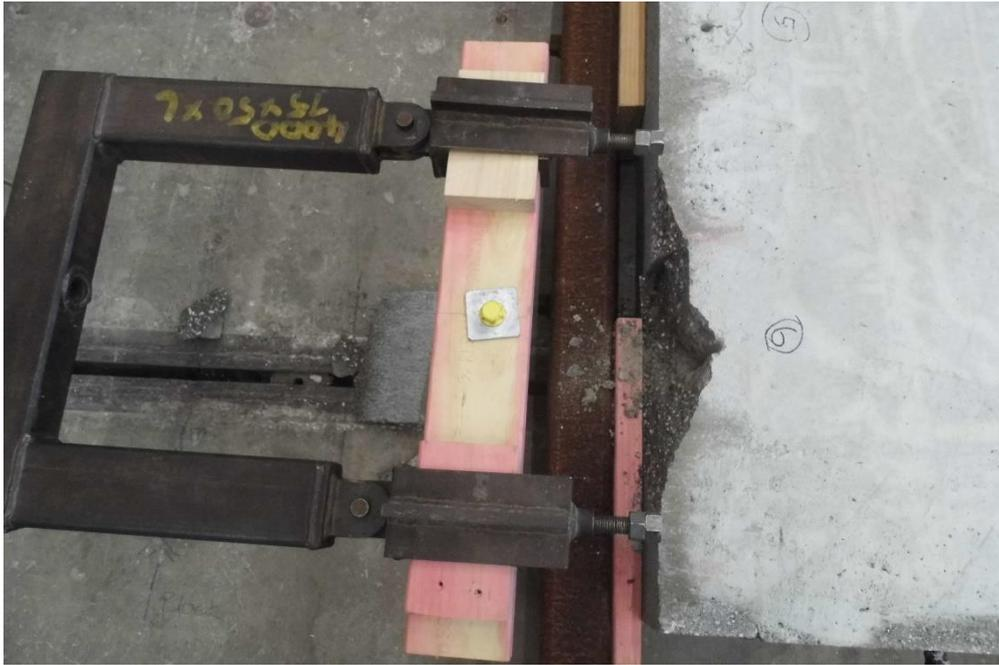
Figure 6. Typical Failure of Out-of-Plane Shear Test Specimens
