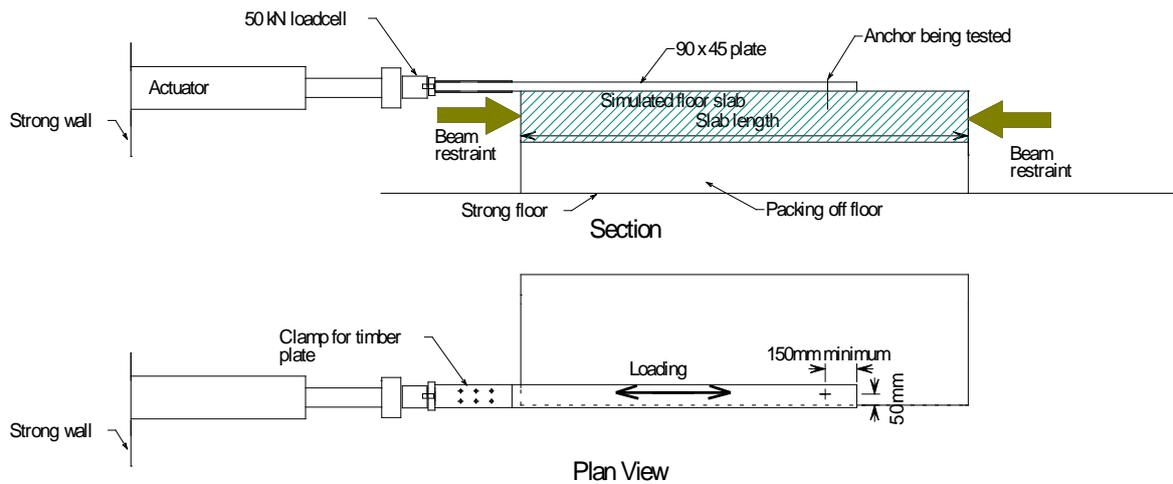
**Figure 2. Test Set-up for Load Parallel to the Bottom Plate (masonry header block form)**
