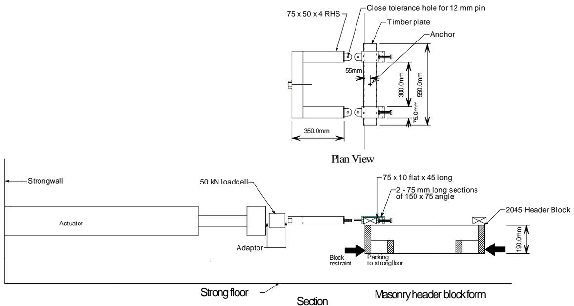
**Figure 3. Test Set-up for Out-of-plane Loading**
