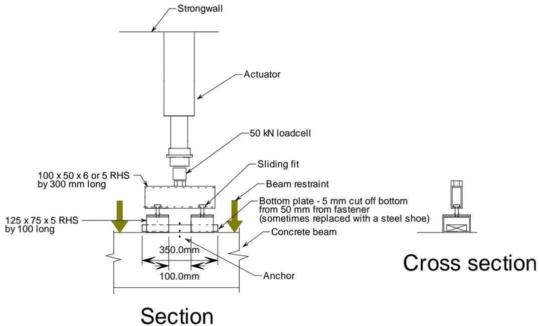
**Figure 4. Test Set-up for Tension Load Testing (Note: Testing Did Not Include Section of Timber, Instead the RHS Section was Directly Connected to Head of Anchor)**
