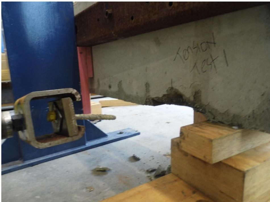
Figure 7. Typical Failure of Tension Test Specimens
