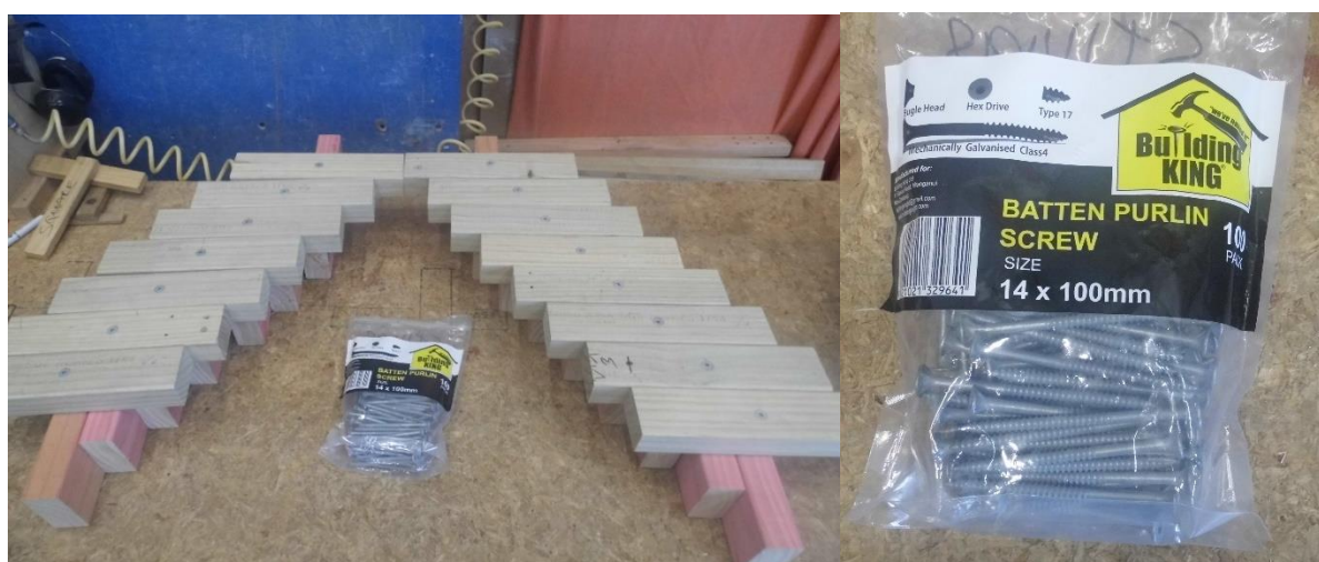
Figure 1. Typical Batten-to-Purlin Connection Specimens and Screw Packaging (Right)
